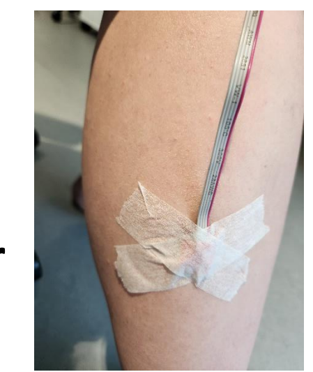
MMG sensor placed on top of muscle belly with medical tape
