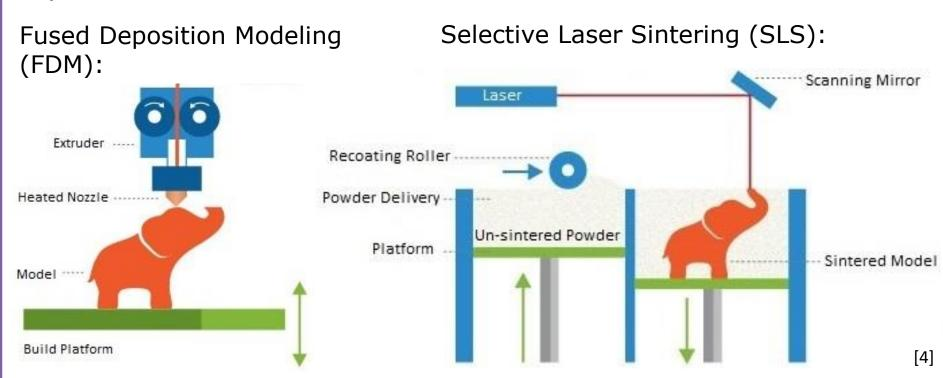
In FDM, layers of melted material are placed on top of each other to build the object one layer at a time. This process has materials suitable for making diagnostic sockets, such as PETG and PLA, as well as definitive ones, such as ABS and PA12.
